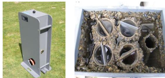
Figure 5. Overview KEMA Biofouling Monitor®
