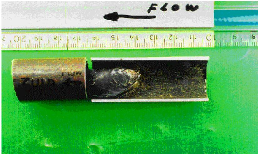
Photo 2: Clamping musselshells were observed inside the tube. Hole is localised under the musselshells.
